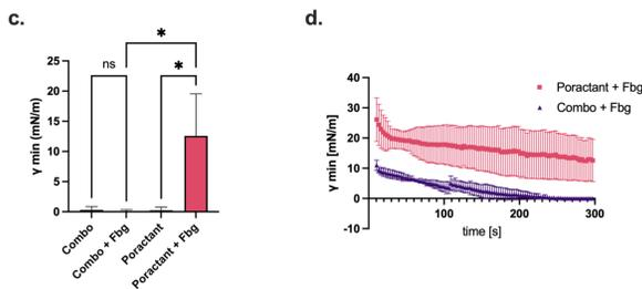
Minimum surface tension ( $\gamma_{min}$ ) of the Combo surfactant and Poractant alfa at concentration 2.5 mg/mL mixed with (a) albumin (Alb) and (c) fibrinogen (Fbg) both at concentration 4 mg/mL after 5 min in PBS.  $\gamma_{min}$  during the whole period of cycling in PBS mixed with (b) albumin and (d) fibrinogen. Data are presented as mean  $\pm$  SD. \* $p < 0.05$ , \*\* $p < 0.01$
